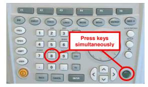
2. Switch the instrument on and keep PRESET and 8 pressed for at least 5 seconds after the startup screen has appeared on the screen.
